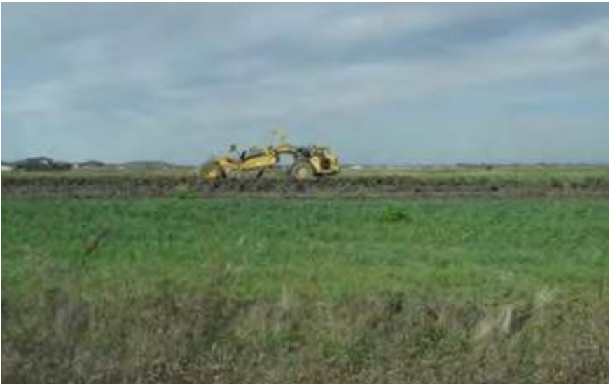
Photo: A Wheel Tractor-Scraper uses a large blade for earth moving.
